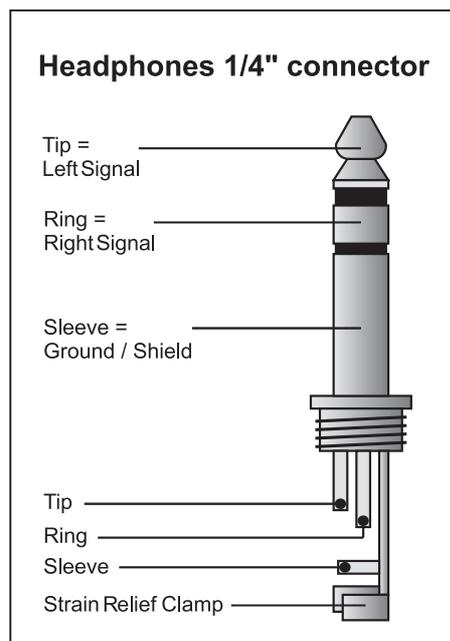
*Fig. 5.2: Wiring of a stereo headphones 1/4" plug*
